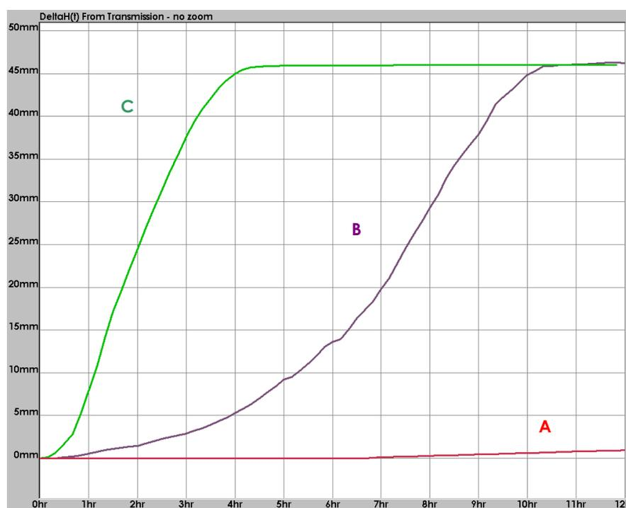
*Figure 2. Thickness of clarified layer for the three ceria suspensions.*
