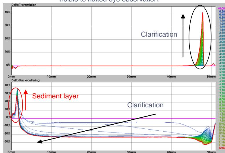
Figure 1. Delta transmission (top) and delta backscattering (bottom) for Ceria suspension A at 35°C.
