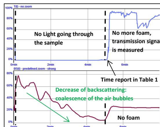
Figure 2: Transmission (top) and Backscattering (bottom) versus time for commercial foam at 30°C
