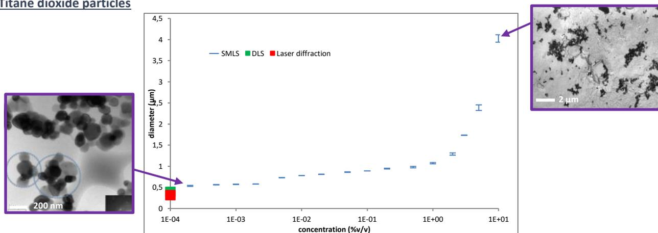
Figure 2: Mean size versus concentration (v/v) for titanium dioxide particles
