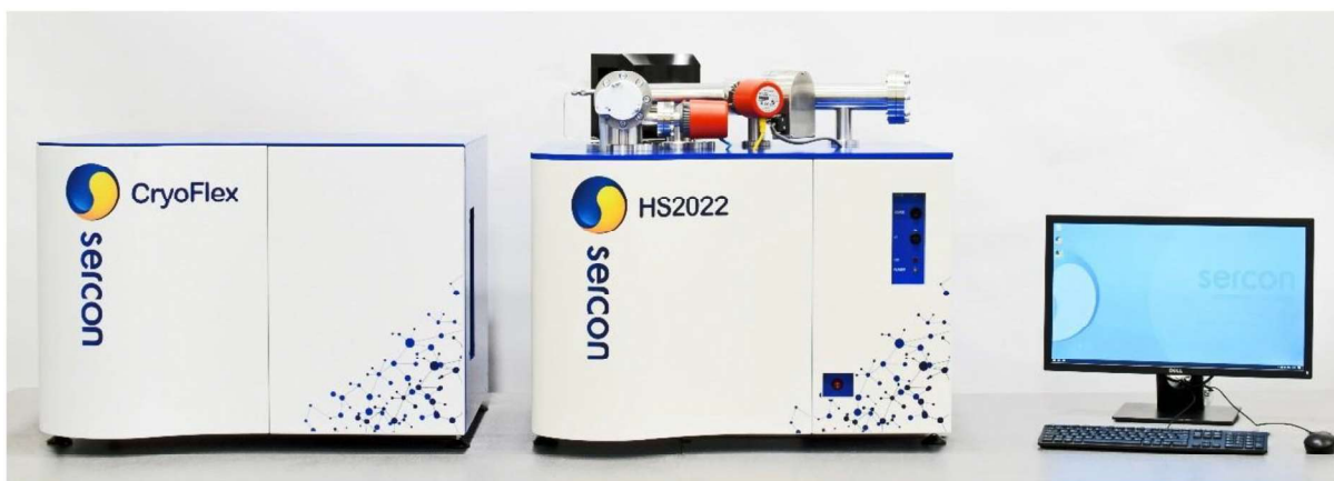
FIGURE 1 The CryoGas 2022 IRMS system. The unit on the left-hand side “CryoFlex” is the basic CryoGas system which has been adapted for CH 4 analysis. This unit contains the GC columns, water CO and CO 2 traps as well as the open Dewar liquid nitrogen system. The unit on the right is the benchtop 20-22 mass spectrometer
